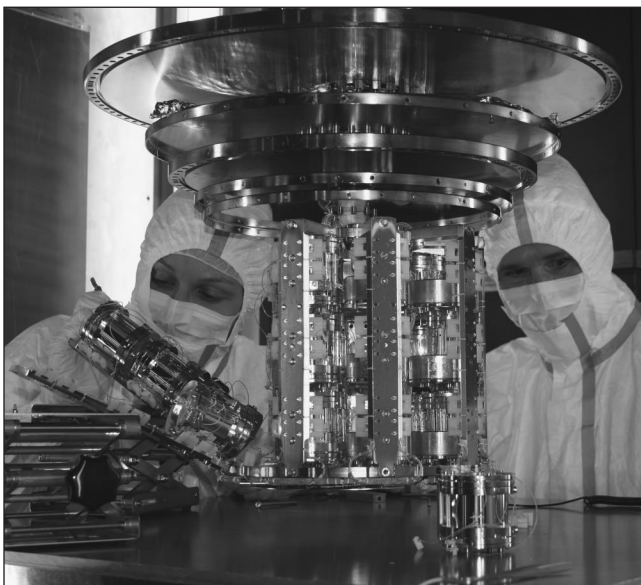
Left: A detector structure that will be used to detect dark matter particles. Each individual cylindrical detector has a \text{CaWO}_4 single crystal, similar to that shown on the bottom right. These crystals are called scintillators, and convert high-energy radiation to light. The Czochralski technique is used to grow the crystal shown on top right, which is a \text{CaWO}_4 ingot. The detector crystal is cut from this ingot.
